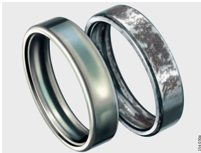
Figure 9 Bearing rings after the salt spray test. Left: a part with Corrotect ® plating; Right: an unplated bearing ring
